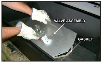
Figure 16.6 Remove Valve Plate
